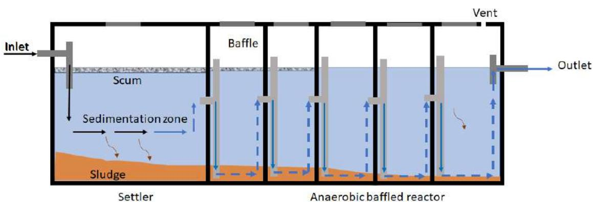
**Figure 4.3.4.** Anaerobic Baffled Reactor septic tank showing location of baffles and three distinct layers (scum (oil, fats, and grease), clarified water, and sludge (Source: Tilley et al., 2014)
