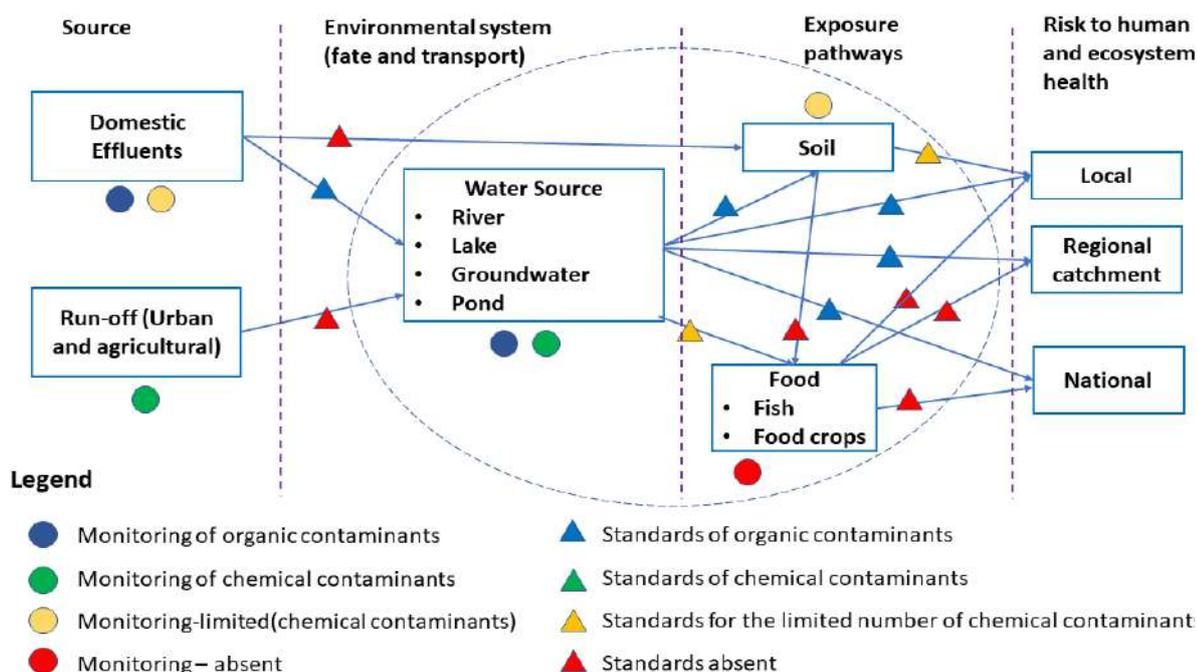
**Figure 3.4.2.** Framework showing gaps in the water quality monitoring framework in India (Adapted from Lele et al., 2021)
