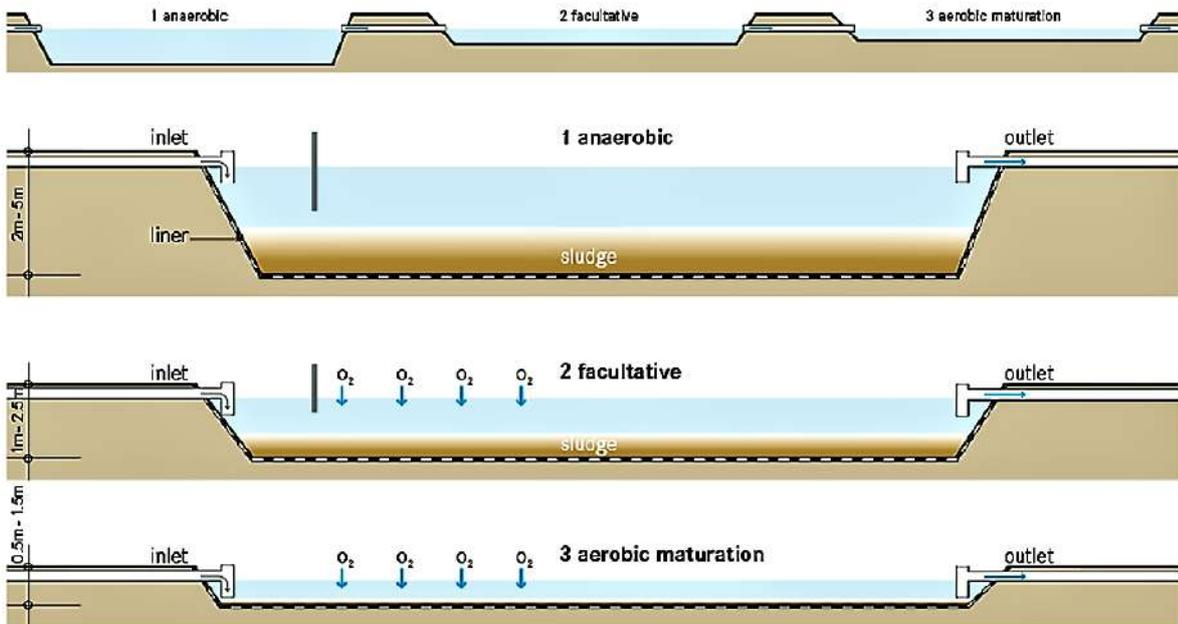
Figure 4.2.7 : Schematic diagram of a waste stabilization system (Source: Tilley et al., 2014)
