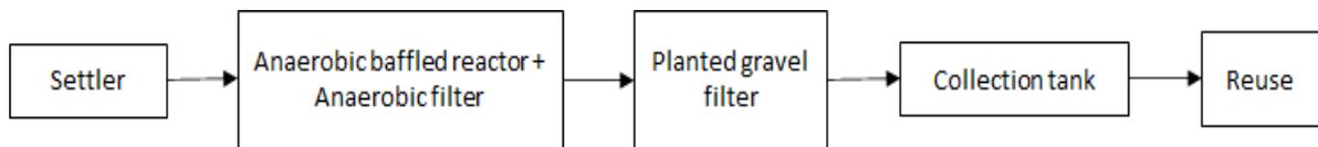
Figure 4.1.1 : Schematic representation of the DEWATS plant of Pune
