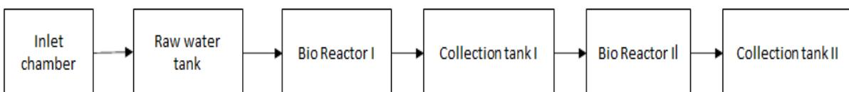
Figure 4.1.2 : Schematic representation of the soil biotechnology unit of Gole Market, New Delhi
